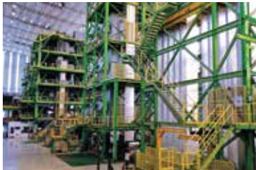
Pickled hot rolled coils are zinc-coated directly (GHR) or after cold rolling (GCR) by continuous hot-dip method on the galvanizing line. Galvanized coating process is applied to both lower and upper surfaces.
