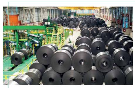
These products are produced by cold-rolling of pickled hot-rolled products.
