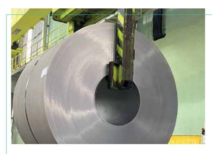
The Pickled and Hot Rolled Products are produced by cleaning the scale layer of hot rolled products with Hydrochloric Acid in the continuous pickling line. Pickled products preferred in places of use where surface cleaning is important in terms of surface appear
